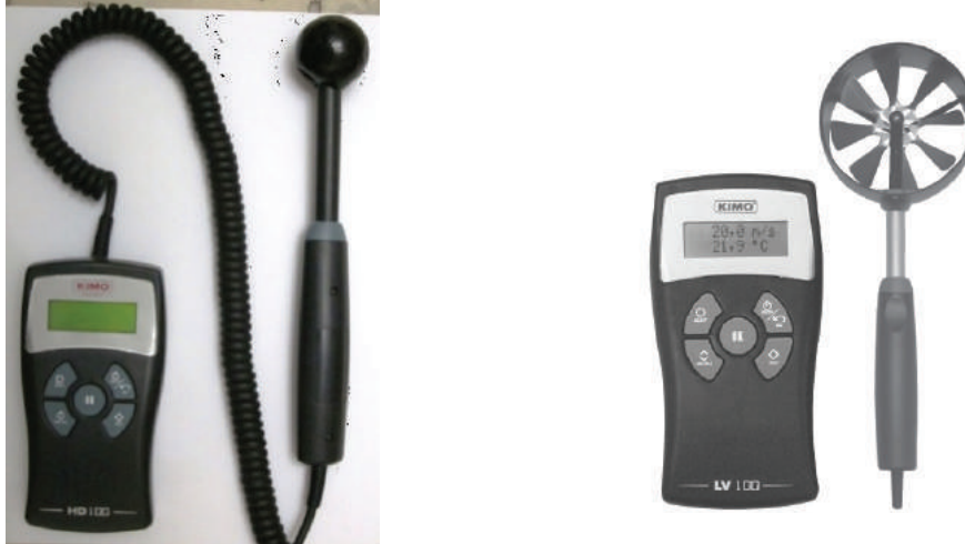
Figura 2 – Left: thermo-hygrometer HD100 Kimo model with a darkened enclosure. Right: thermo-anemometer LV100 Kimo model. Fonte: Author, 2014
